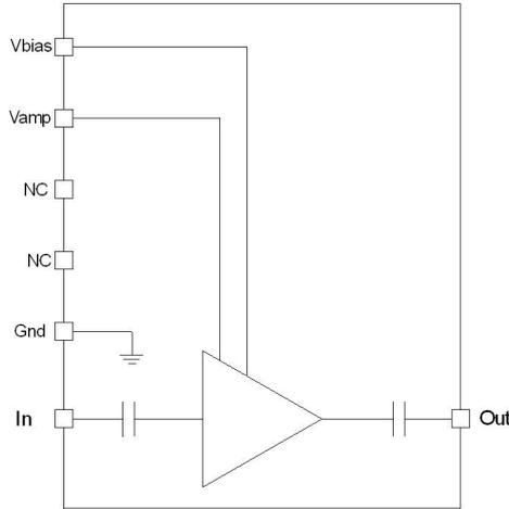
Mechanical Diagram and Pinout
